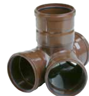
HS®-Junction Base K90 with lateral inlet 45°
