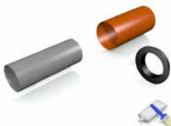
Position pipe ends.
